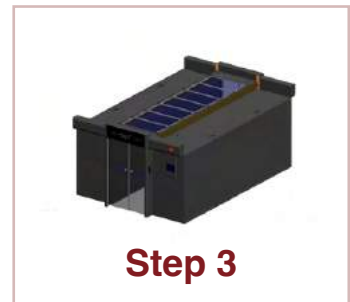
End door installation
